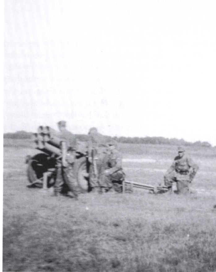
Waffen-SS troops with a Nebelwerfer during a lull in the fighting. The electrical cable that led to the remote firing mechanism can be just seen running from the gun tube between the two wheels. The Nebelwerfer was mounted on the same carriage as that of the 3.7cm PaK35/36.
