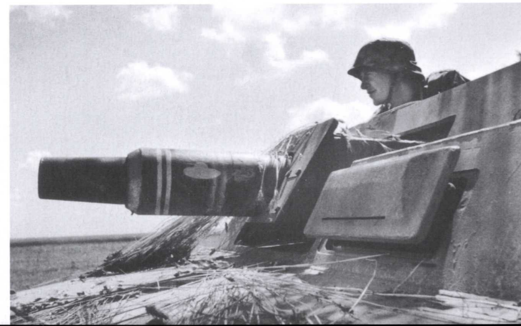
A Waffen-SS Sd.Kfz.251 halftrack armed with a 7.5cm short gun barrel of a Pz.Kpfw.IV during operations at Kursk in July 1943. Note the white painted kill rings on the barrel of the 7.5cm gun.
