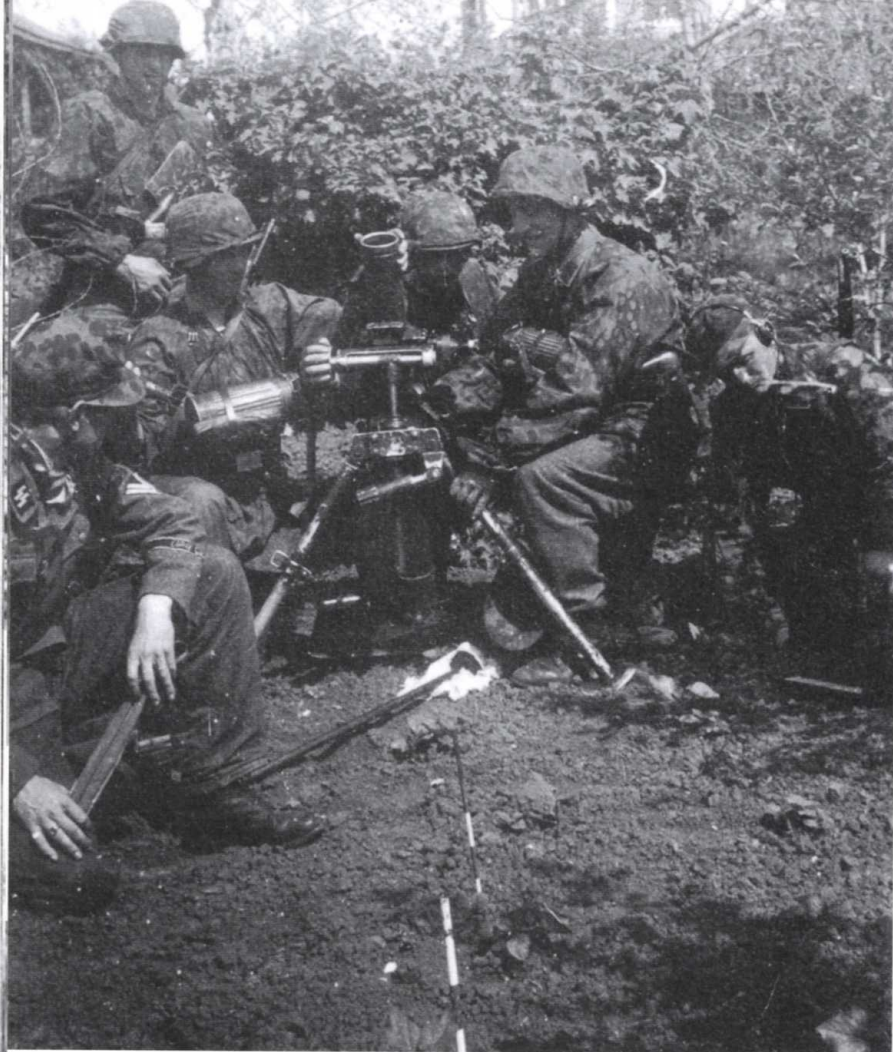
Two photographs showing Waffen-SS and Wehrmacht mortar crews with the standard German mortar was the 8cm Granatwerfer 34 or Gr.W.34 mortar. The mortars maximum range was 2.4km when it fired the standard Wurfgranate 34 round which carried 550g of explosives. The round could be set to detonate on impact or in an airburst. It could also fire the Wurfgranate 40, a larger round with an increased explosive charge of almost 5kg. However this decreased the maximum range to 950m.
