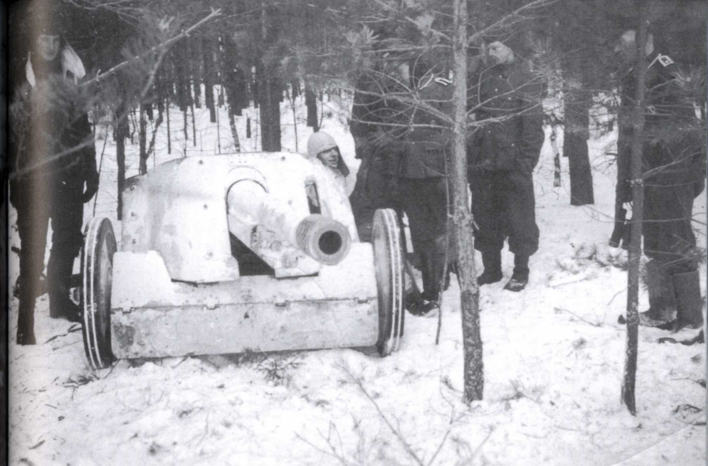
Well concealed inside a wooded area the crew of white-washed 7.5cm PaK40 can be seen with their deadly anti-tank weapon. The PaK40 had spaced-armour shield which was held together by large bolts. These bolts also had drilled holes that allowed the crews to thread foliage through them.
