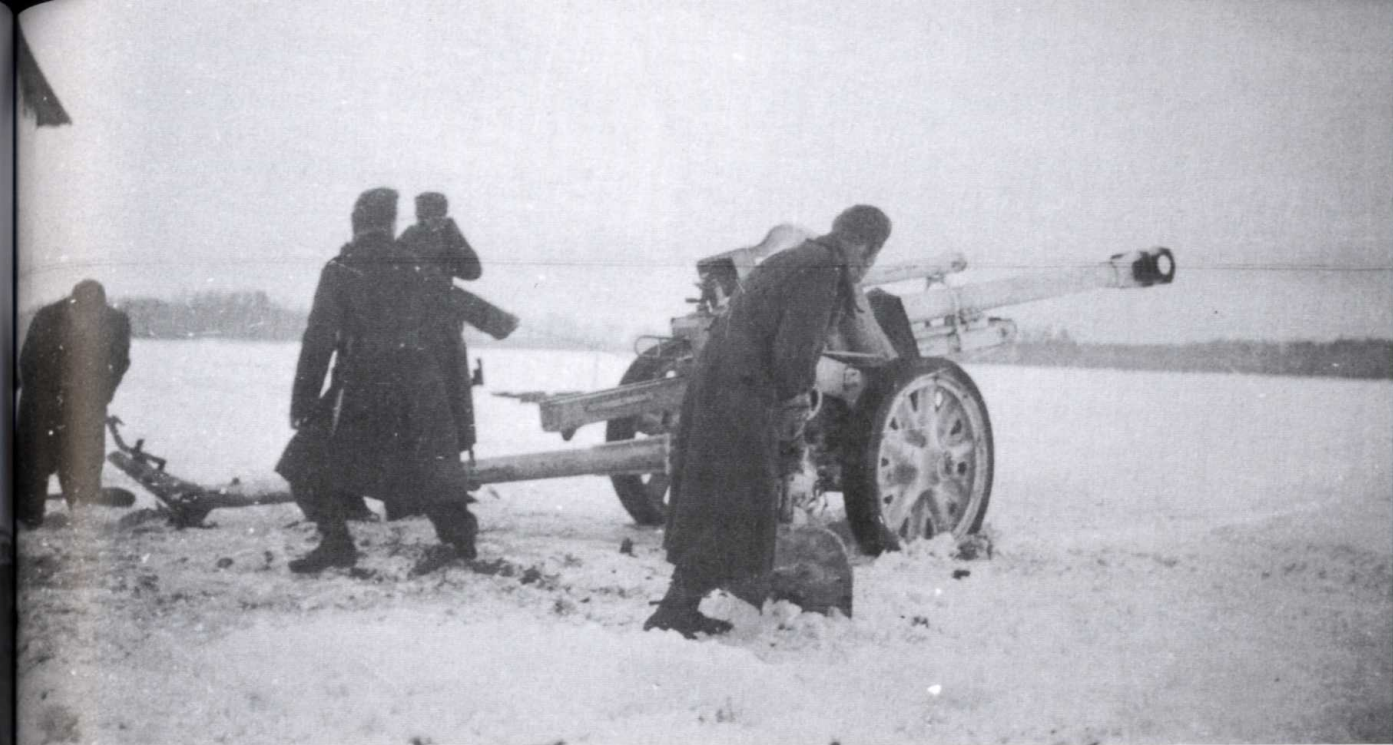
A photograph taken the moment a modified 10.5cm le FH 18/42 is fired against an enemy target during fighting in Army Group Centre in early 1944. The gun has received an application of winter white wash paint and blends well with the local terrain.
