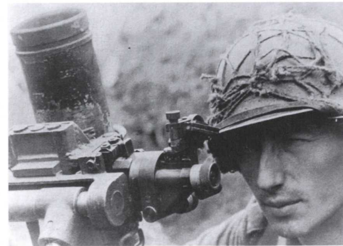
Four photographs showing an 8cm sGrW 34 mortar in action against an enemy target. Each battalion fielded some six of these excellent 8cm sGrW 34 mortars, which could fire 15 bombs per minute to a range of 2,625 yards. Aside from high-explosive and smoke bombs, this weapon also fired a "bounding" bomb. It was very common for infantry, especially during intensive long periods of action, to fire their mortar from either trenches or dug-in positions where the mortar crew could also be protected from enemy fire.
