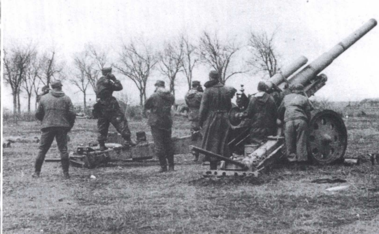
A number of Wehrmacht troops plug their ears as the 15cm field howitzer is about to be fired. Note the trail spades dug into the ground. These were designed to help prevent the full impact of the howitzer's recoil after firing and reduce the backward movement of the gun.
