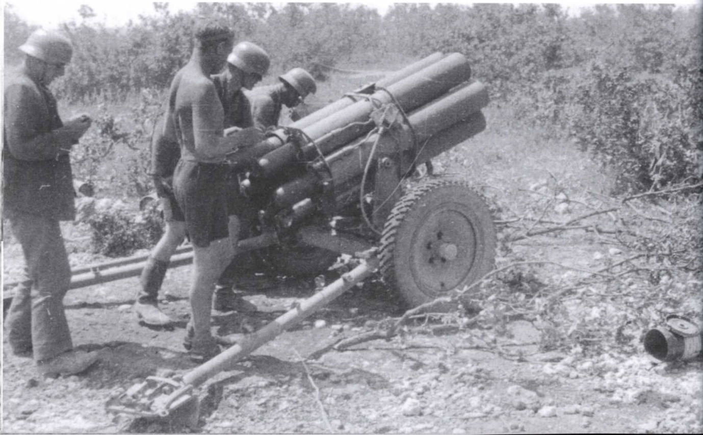
Two photographs showing the 15cm Nebelwerfer 41 being prepared for firing and launching the deadly six-barrelled rocket launcher into action. This weapon fired 2.5kg shells that could be projected over a range of 7,000 metres. When fired the projectiles screamed through the air, causing the enemy to become unnerved by the noise. These fearsome weapons that caused extensive carnage at Kursk served in independent army rocket launcher battalions, and later in the war in regiments and brigades.
