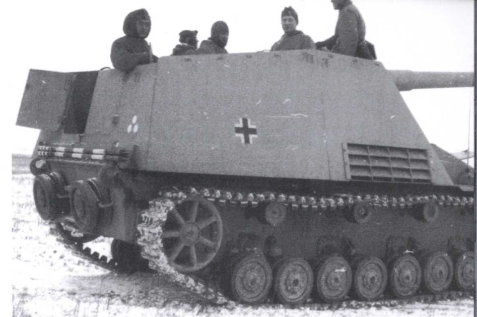
The crew of a Hummel self-propelled gun wearing the reversible parka grey-side out have halted in a field with a battery of Hummel's during a defensive action in very early 1944. The Hummel mounted the standard 15cm heavy field howitzer in a lightly armoured fighting compartment built on the chassis of a Pz.Kpfw.III/IV.
